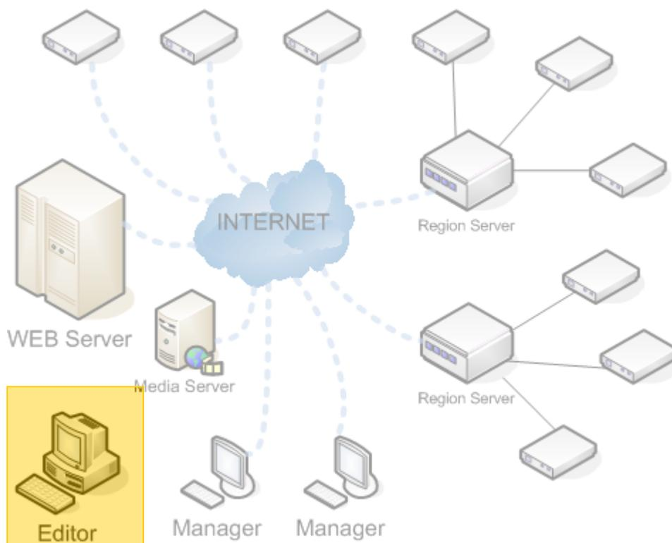
The editor is used for editing the contents of program to define the media's show period and order. In the same time, the editor contains package-export function, which can pack all contents into a separate package after edited; the package can be distributed to all terminals through the network or by manual to achieve the distribution of programs.
