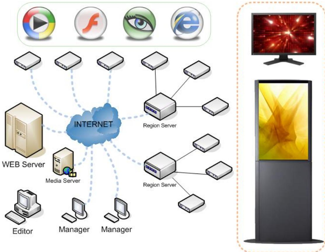
All terminals in this system are monitored and managed by a WEB server, and only need to be connected in the Internet, and then they will communicate with the WEB server automatically. All terminals will feedback their current state to the server regularly, and receive the program files for automatic timing display.
