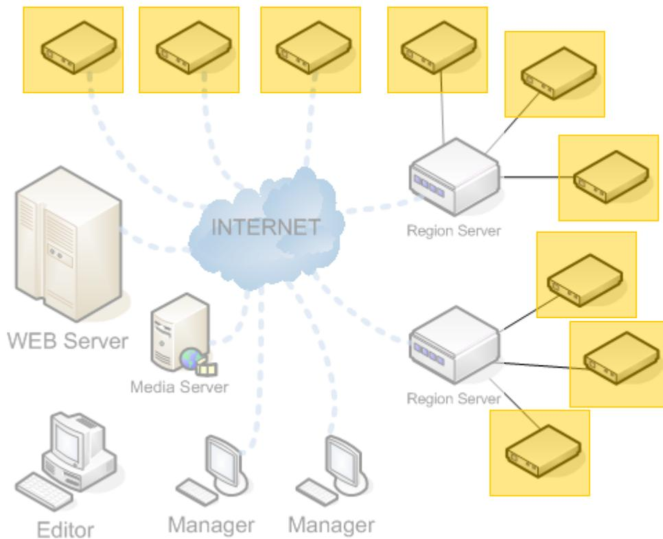
Terminals can run on X86, ARM, MIPS hardware environment by using the Linux operating system. They can segment the output screen into many sub-regions which play different contents by the method defined in program.
